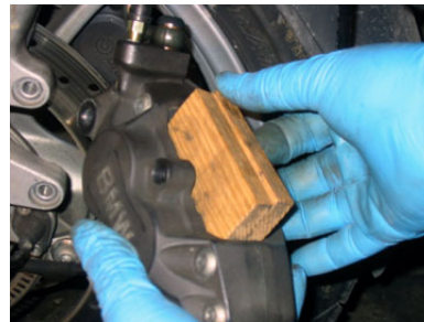
Front pistons being pushed back and blocks inserted.
