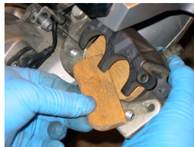
Rear pistons being pushed back and blocks inserted.
