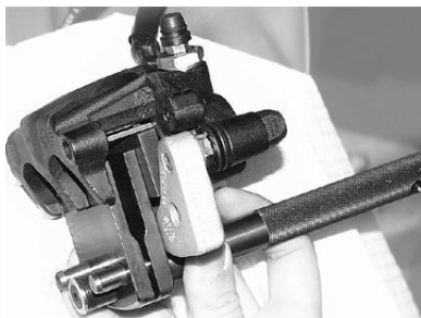
Rear pistons being pushed back.
