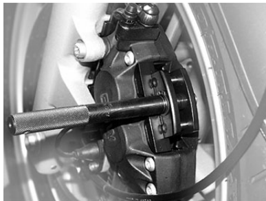
Front pistons being pushed back.
